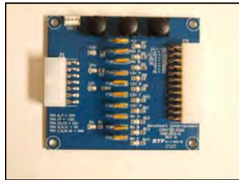
Power Distribution PCB
