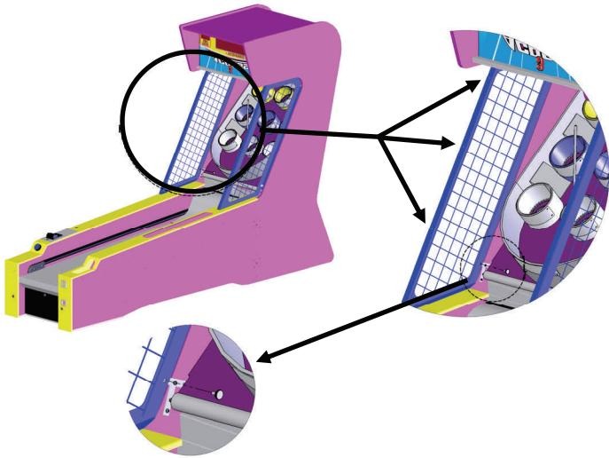
8. There are 3 thumb screws on each side to connect the front cage and two bottom screws to hold the sides.
