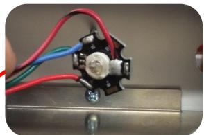
+5 volt LED Lights are mounted with the red w/brown wire loop at the top, over the mounting screw. HAND TIGHT PLASTIC NUTS!
