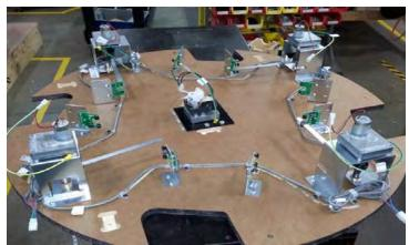
You now have access to the turntable motor, the arm motors, the win spot motors/RFID and the player button assemblies.
