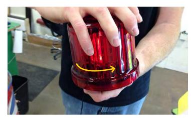
Plug in the beacon cable at the top of the marquee and place the beacon so that the red button is aligned with the cut out area (button should NOT be pressed in).
