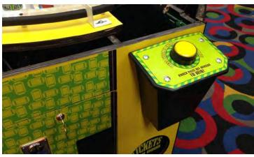
Plug in the buttons, grounds and speakers as shown. Insert the button switch into the button housing and turn, locking into place.
