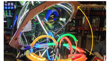
Lift the dome from the Red side; it will hinge back and rest in an open position.
