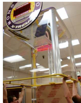
Set Top Assembly onto Base
