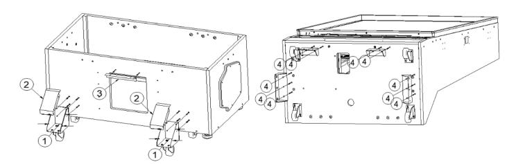
B. Put Main and Bottom case end to end and secure both cases as shown below.
