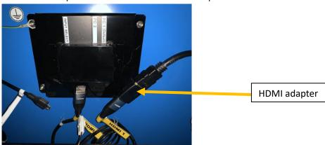
5. Power on the machine. The video displayed on the top monitor will now ALWAYS be from PC1. If needing to view PC2 image, simply remove HDMI 1 from the adapter and plug in HDMI 2.
