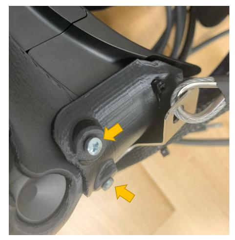
4. Refasten the cable cover screws prior to tightening the cable tie.
