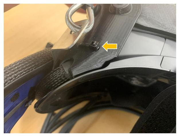
**REASON FOR THE CHANGE:** Some operators have experienced intermittent laggy video on the top monitor and loss of video in the headsets. This has been determined to be caused by either a loose or failed All-in-One cable. This modification will remove the possibility of a loose cable at the headset connection.
