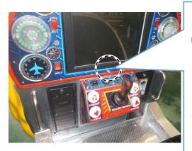
Open the monitor frame using key #711, Monitor will automatically raise up slowly by gas spring. Inside, you will find the Main PC and I/O as well as other components.
